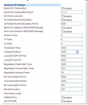
The "XML SIP Notify" field is disabled by default. To enable this field, check the box.
