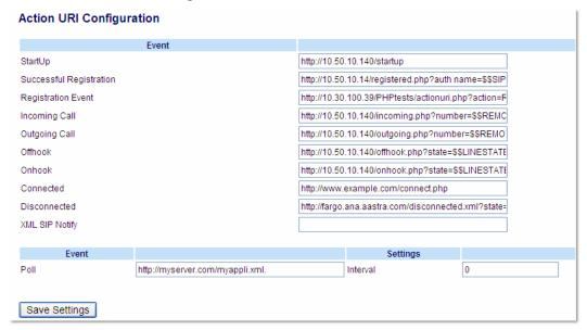
2. In the "Disconnected" field, enter a valid URI for which the phone executes a GET on, when it transitions from the incoming, outgoing, calling, or connected state into the idle state. Leaving this field empty disables the Action URI Disconnected feature. For example,
