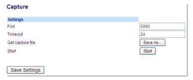
2. In the **Port** field, enter the port or ports from where the phone should capture traffic (e.g. 5000:6000;7000).
