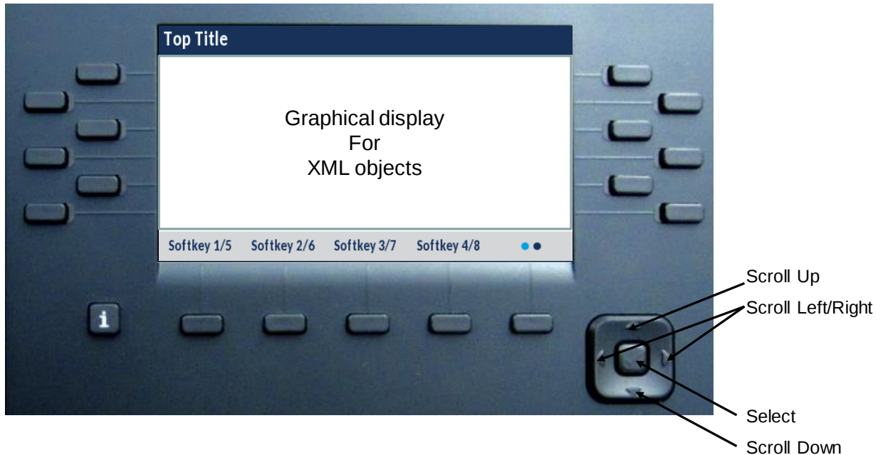
Figure 12: Mitel 6869i XML display and keys
