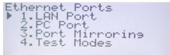
6. With **LAN Port** highlighted, press the up and down navigation key to navigate to the selected column and press Enter. Use the up and down navigation key to select the desired speed and duplex method and press the right navigation key to Save the selection. Applicable values include:
