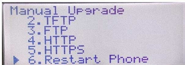
To configure connection settings for a manual upgrade of 6920, 6930 and 6940 IP Phones:
