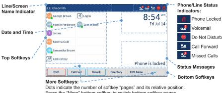
Dots indicate the number of softkey "pages" and its relative position. Press the "More" bottom softkey to switch bottom softkey pages. Swipe left and right in the top softkey area to switch top softkey pages.
