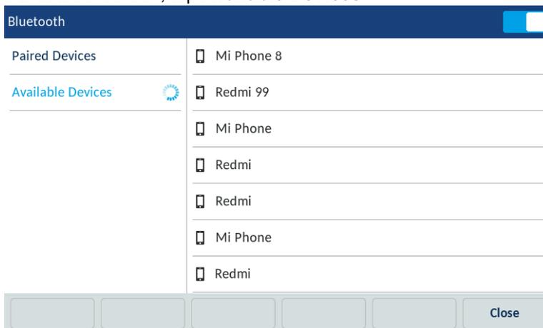
**Note:** The Mitel 6970 IP phone scans for supported Bluetooth mobile phones when viewing the list of available devices. Refer to the respective Bluetooth mobile phone documentation for discovery and pairing procedures that must be performed on your Bluetooth mobile phone.
