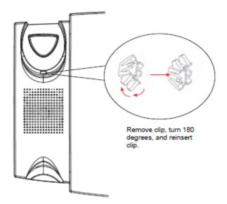
**6.** Place the handset into the phone's cradle, inserting the legs on the clip into the square hole on the handset. This allows the handset to rest in the cradle in a vertical position without slipping off when the phone is installed on the wall.
