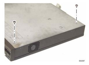
**6.** Screw the supplied small bracket onto the bottom of the controller as shown.
