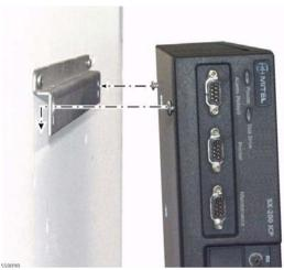
**9.** Insert a screw into the bottom bracket to stabilize the controller as shown below.
