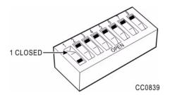
The S1 switch settings on the PRI Card shown in the following illustration inform the T1 module of the location of the clock source and must be set as indicated.
