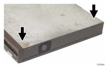
3. Remove the two feet as shown below.
