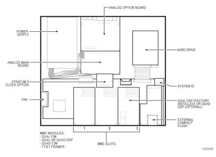
Figure 5: Controller Components
