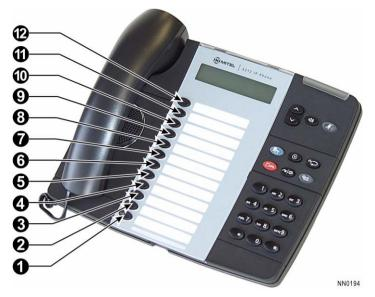
The programmable keys on 5224, 5324 and 5340 (5324 and 5340 not shown) IP Phones are numbered as follows: (see Note)
