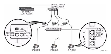
Figure 6: Power Brick Connections for 5200 Series IP Phones
