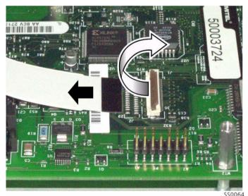
6. Remove the internal flash card as shown in the following figure.
