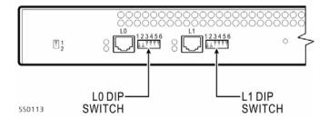
Figure 9: NSU DIP Switch Location
