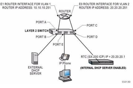
Figure 19: VLAN Configuration 1
