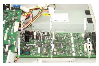
**8.** Remove the two screws at the back of the unit as shown in the following figure.
