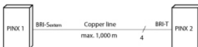
Figure 31: BRI-S basic rate interface external, networked with copper line
