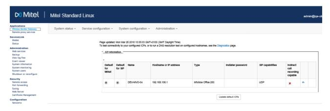
Ensure the 'Hostname or IP Address' setting used for the ICP matches the IP Address configured for the Node on the MCS server.
