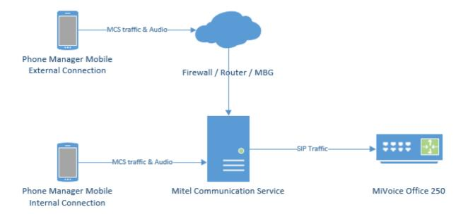
The MCS SIP Proxy requires G.711 to be configured against the SIP Endpoint on the telephone system as the audio encoding for making calls.
