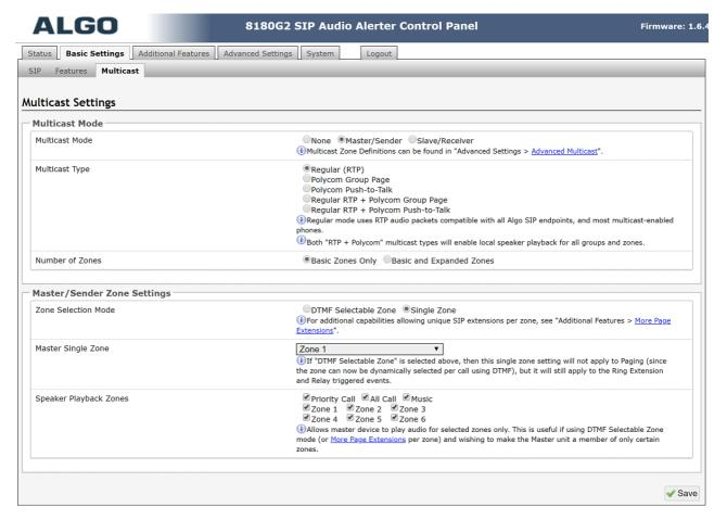
Using a paging unit in 'Master/Slave' mode allows MiNET/Digital extension to page 69xx units.
