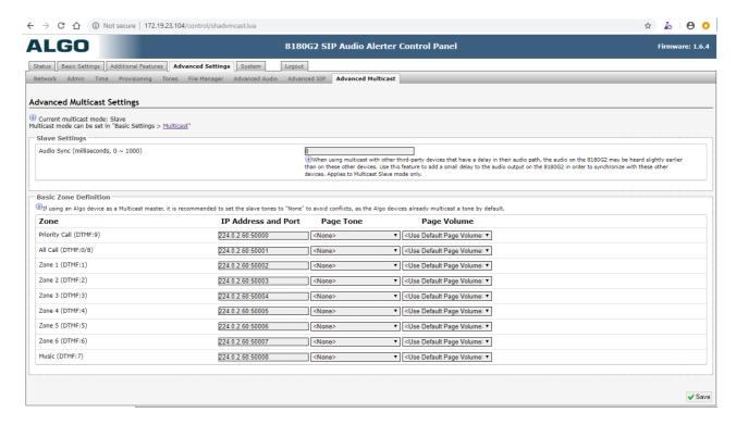
Once configured, 6900 series phones will be able to page directly to the Algo SIP paging unit over multicast, with no SIP registration with the MiVoice Office 250 necessary.
