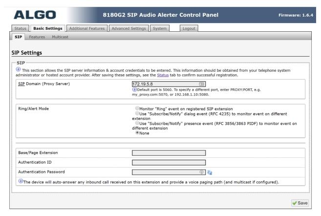
To use the paging unit in this manner, create a SIP extension on the telephone system and then add the extension, authentication ID and password on the 'Basic Settings\SIP' tab.
