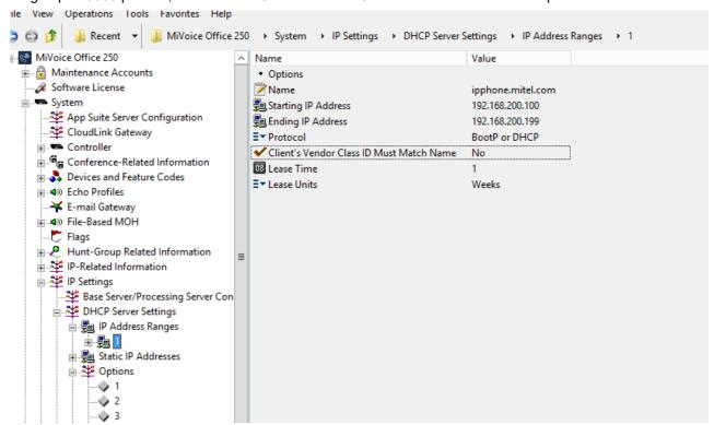
Removing the Vendor Class ID matching will cause all devices (including computers) to receive DHCP addresses from the MiVoice Office 250.
