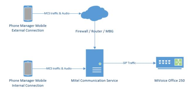
The MCS SIP Proxy requires G.711 to be configured against the SIP Endpoint on the telephone system as the audio encoding for making calls.
