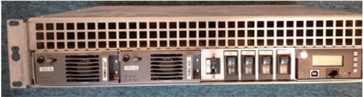
Figure 3.6: 2U height AC/DC Power Unit, 800-1600W
