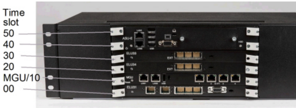
Figure 3.2: MX-ONE Lite, 87L00039BAA-A, equipped with MGU2, ASU and 3 additional boards
