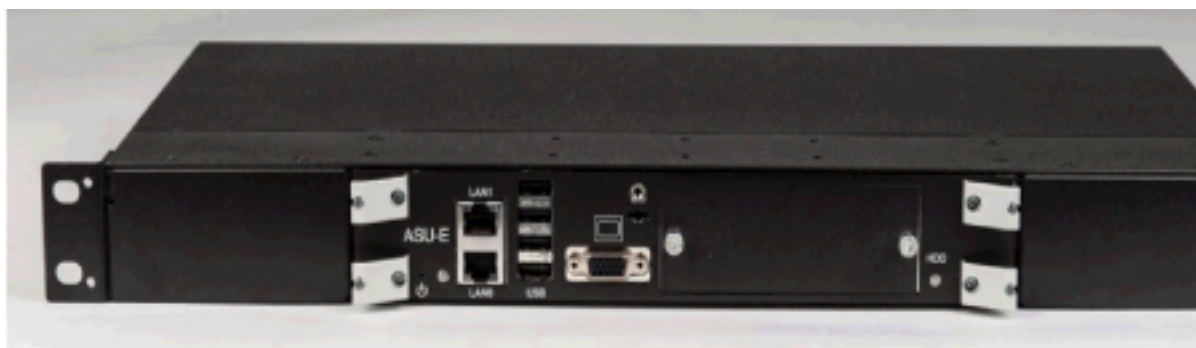
Figure 3.5: ASU in a MX-ONE 1U chassis
