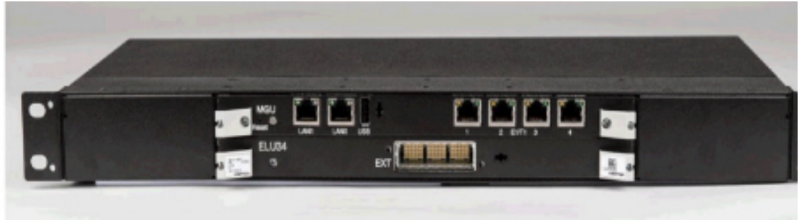
Figure 3.1: The MX-ONE 1U chassis equipped with MGU2 and ELU34
