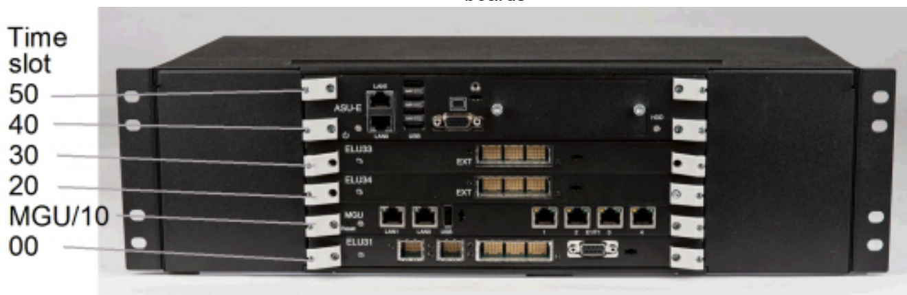
Figure 3.2: MX-ONE Lite, 87L00039BAA-A, equipped with MGU2, ASU and 3 additional boards
