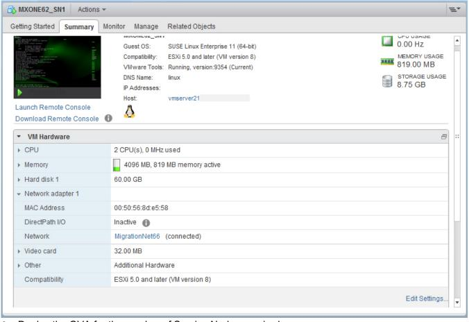
Figure 4.11: Verification of the MX-ONE VM setup
