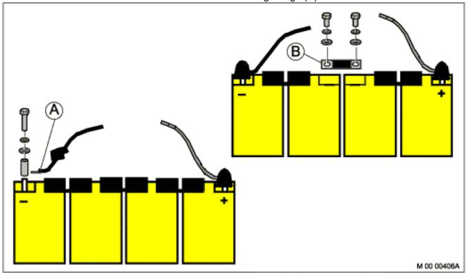
Figure 3.58: Example of Removing the Negative Battery Conductor (A) and an Interconnecting Bridge (B)
