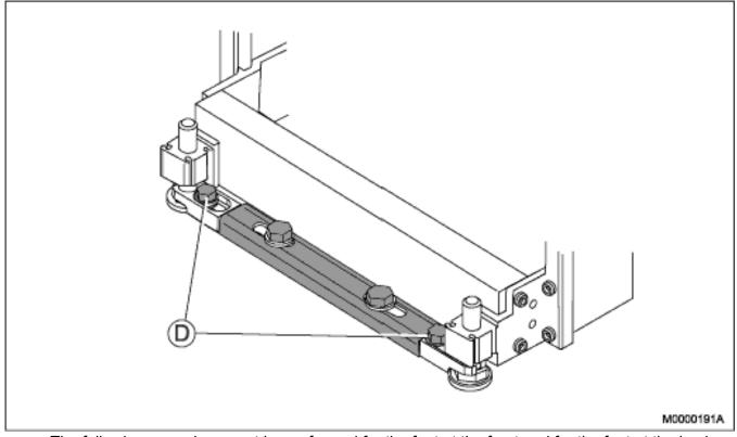
Figure 3.21: Securing the Earthquake Bracing
