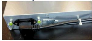
Figure 3.43: Secure Main cables
