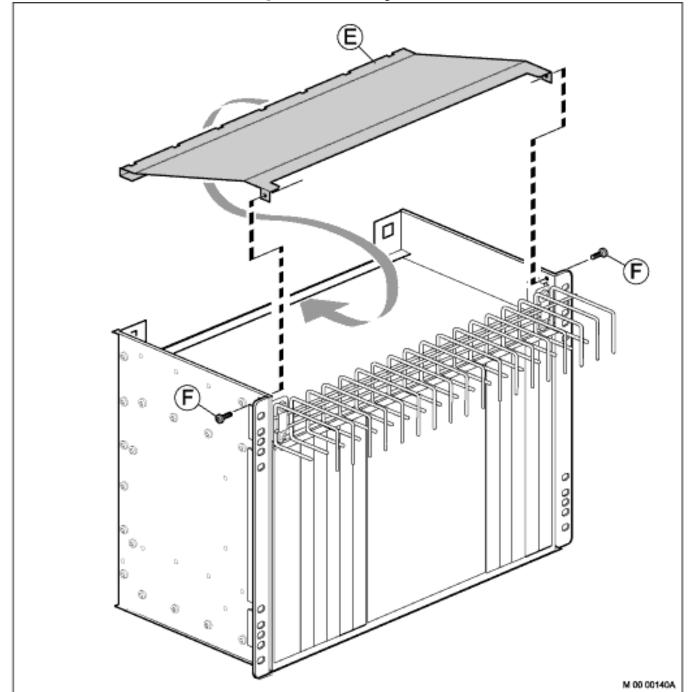
Figure 3.33: Mounting the Lower Air Plate
