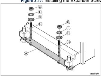
Figure 3.17: Installing the Expander Screw
