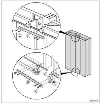
Figure 3.13: Mounting the Earth Bar
