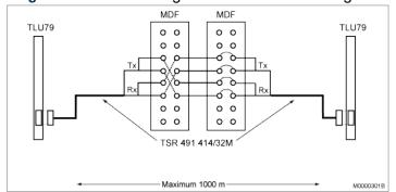
Figure 3.76: Connecting TLU79 to TLU79 through MDF (8 pairs)
