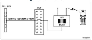
**NOTE:** ELU31/4 can today be used in /3 or /4 mode. Check that the switch, both poles, are in correct position.
