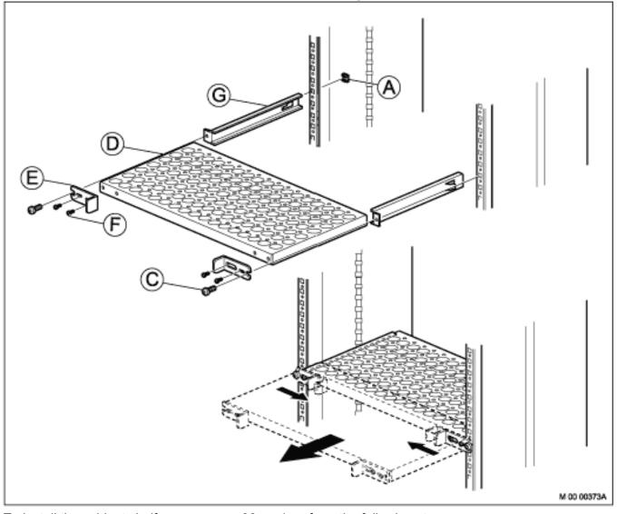
Figure 3.45: Installing Cabinet Shelf
