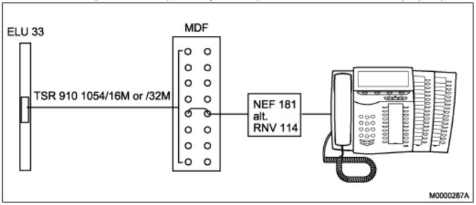
The installation instructions 1/LZT 102 537 and 1/LZT 102 762 show how the wires are connected to terminal block NEF 181 or RNV 114. Regarding connection of system telephone DBC 2xx:
