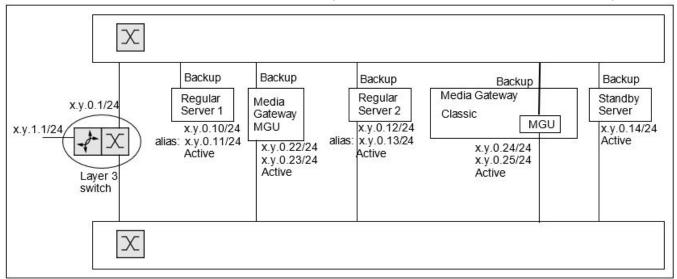
Figure 1.24: Server redundancy with Ethernet bonded network redundancy
