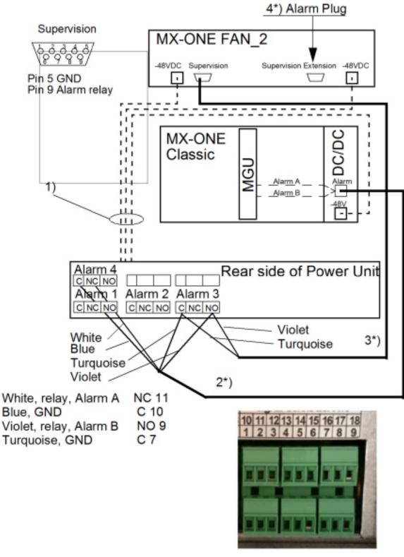
Figure 3.81: Power and Fan alarm in Classic chassis
