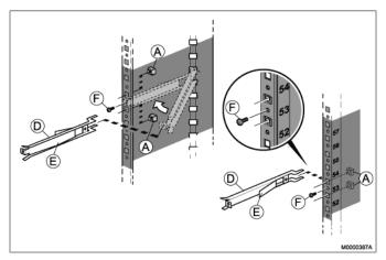
Figure 3.41: Installing the Fan Unit
