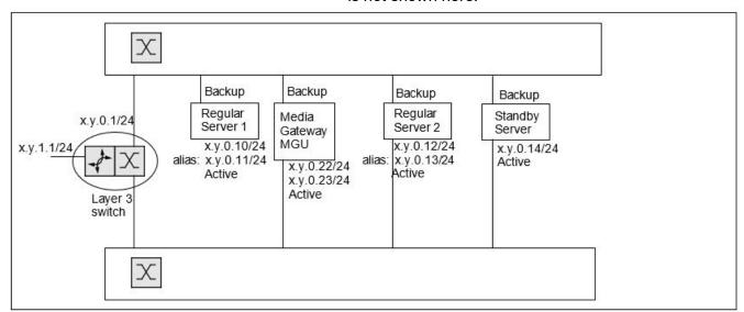
**Figure 1.2:** Server redundancy with Ethernet bonded network redundancy. System database is not shown here.
