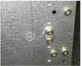
Figure 3.32: Earthing point 7U-chassis
