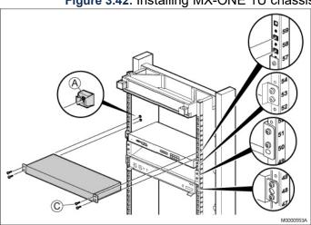
Figure 3.42: Installing MX-ONE 1U chassis
