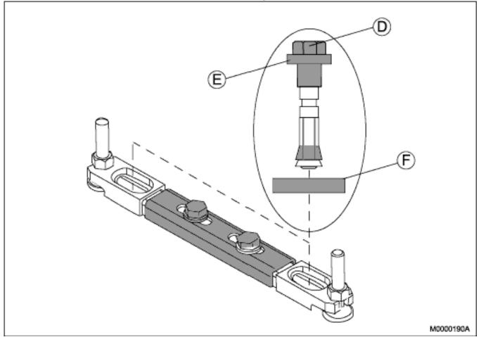
Figure 3.20: Installing the Expander Screw
