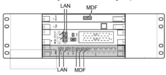
Figure 3.63: MX-ONE Lite cabling example
