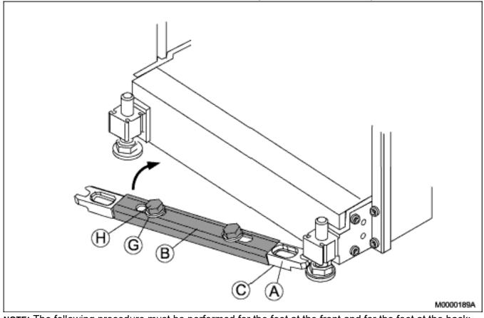
Figure 3.19: Installing the Earthquake Bracing
