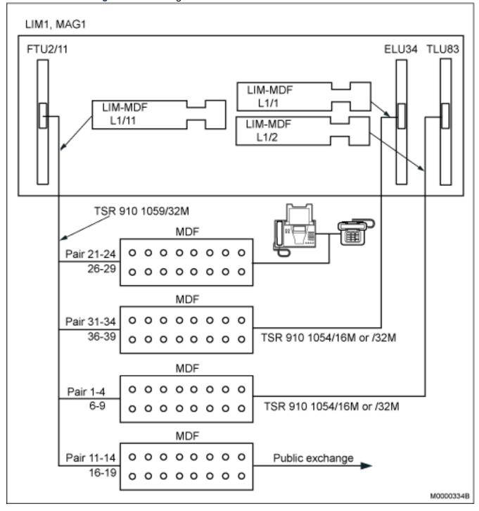
Figure 3.77: Through-Connection on Power Failure or Processor Malfunction
