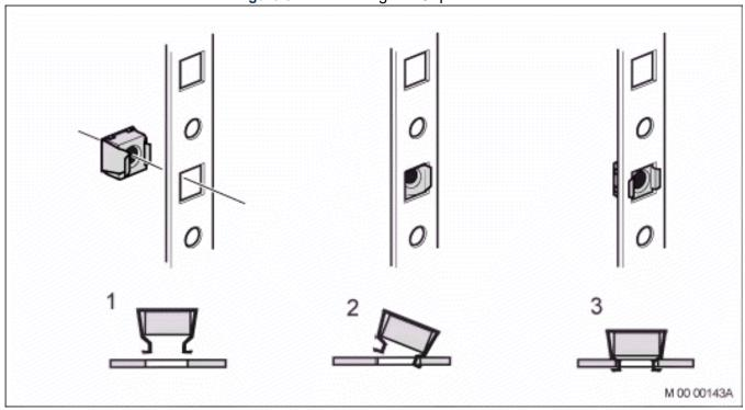
Figure 3.24: Mounting the Captive Nuts in the Rack
