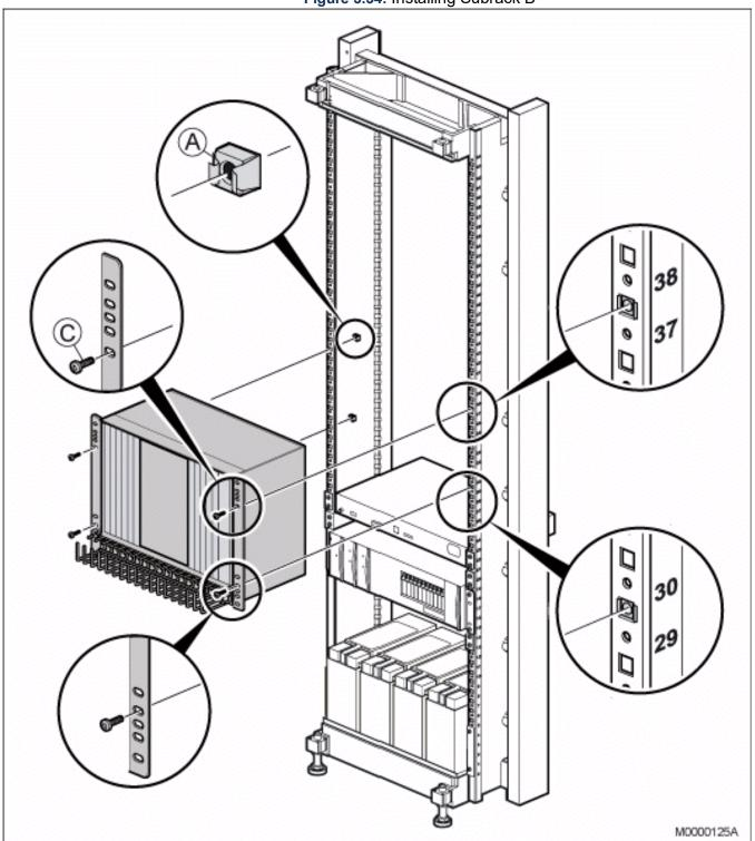
The lower air plate is only mounted in subrack B (lower subrack if two subracks are mounted onto of each others), see Mounting the Lower Air Plate on page 26. In subrack A (upper subrack), front and rear air plates are installed instead.
