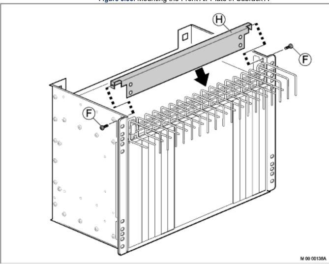
Figure 3.35: Mounting the Front Air Plate in Subrack A
