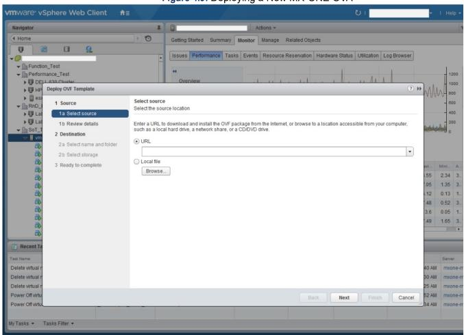
Figure 4.9: Deploying a New MX-ONE OVA
