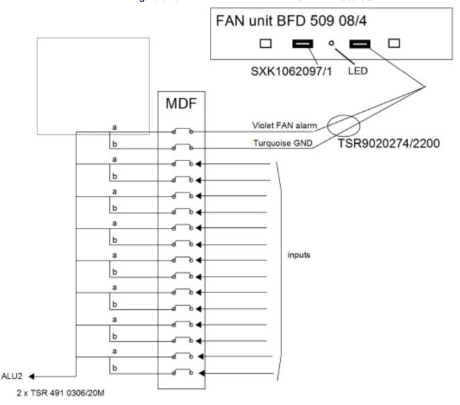
Figure 3.79: MDF Alarms for the Fan Unit BFD 509 08/4
