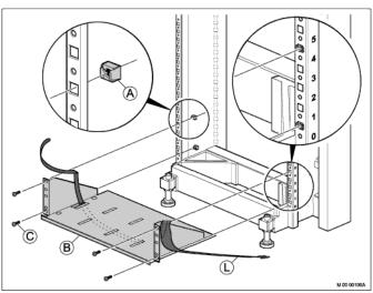
Figure 3.25: Installing the Battery Shelf
