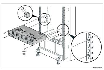
Figure 3.30: Installing AC/DC Unit
