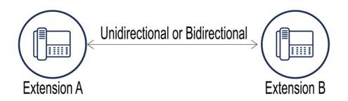
Mitel supports unidirectional or bidirectional one-to-one ringdown.
