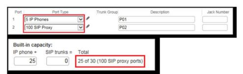
Figure 13: Port Allocation Designated on Switches
