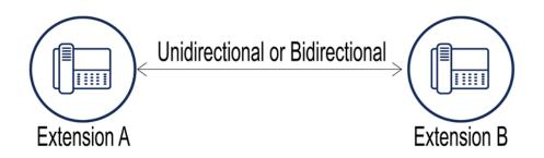
Mitel supports unidirectional or bidirectional one-to-one ringdown.
