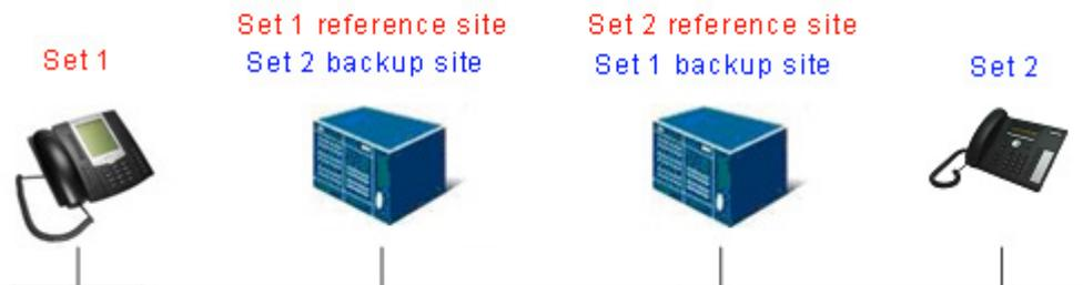
This example illustrates the case in which each site serves as backup for the subscriptions on the other site. This architecture is primarily used in cases where the multi-site configuration involves only 2 sites.
