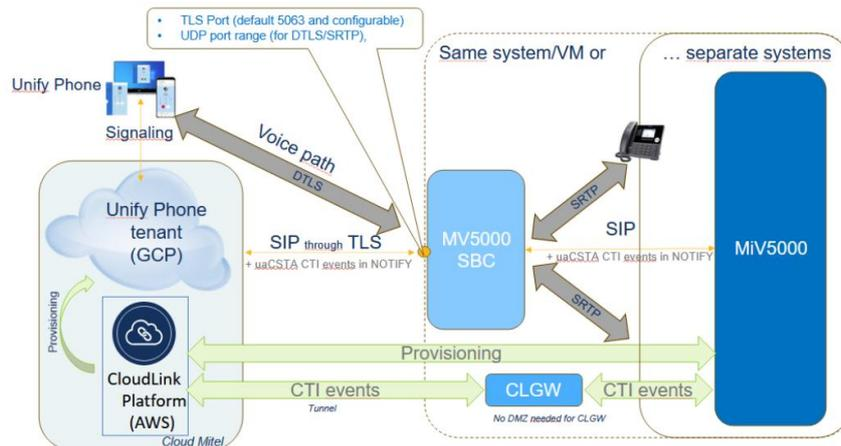
A standard configuration is recommended for Unify Phone. The Daisy Chain configuration is possible. For more information about the possible configurations with the SBC, refer to the paragraph **2.3 – SBC Service architectures**.
