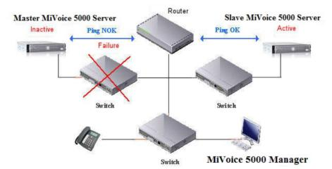
The master MiVoice 5000 Server PC was deactivated upon a ping NOK. The slave MiVoice 5000 Server PC became active after 10 seconds of network failure.
