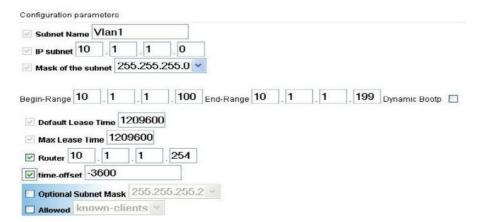
The **upper part** defines the **specific network parameters negotiated via option 43** with the terminals for the subnet in question.
