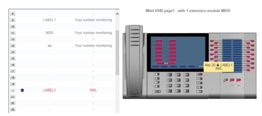
Clicking **Page 2** (in the example) at the bottom of the extension displays the numbers of the first to last key on Page 2 of the extension so they can be programmed.
