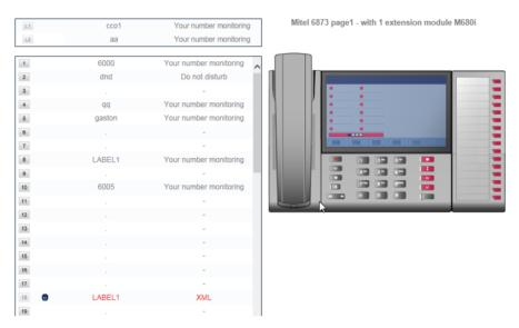
Clicking **Next** on the terminal displays the numbers of the first to the last key so they can be programmed.
