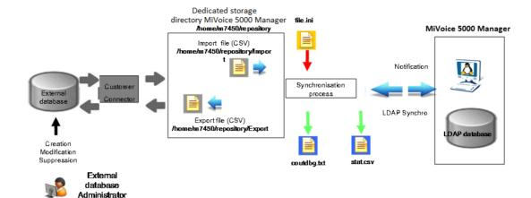
The principle is to synchronise the external directory database and the MiVoice 5000 Manager LDAP database by exchanging description files in .csv format in **UTF-8 without BOM**.
