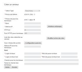
For an external download server integrated into MiVoice 5000, the integrated TMA in MiVoice 5000 Manager uses the MiVoice 5000 Manager account to copy the files (configuration software and files) from the TMA directories to the integrated download server directories.
