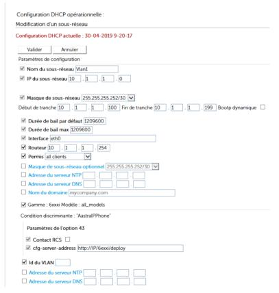
The **upper part** defines the **specific network parameters negotiated via option 43** with the terminals for the subnet in question.
