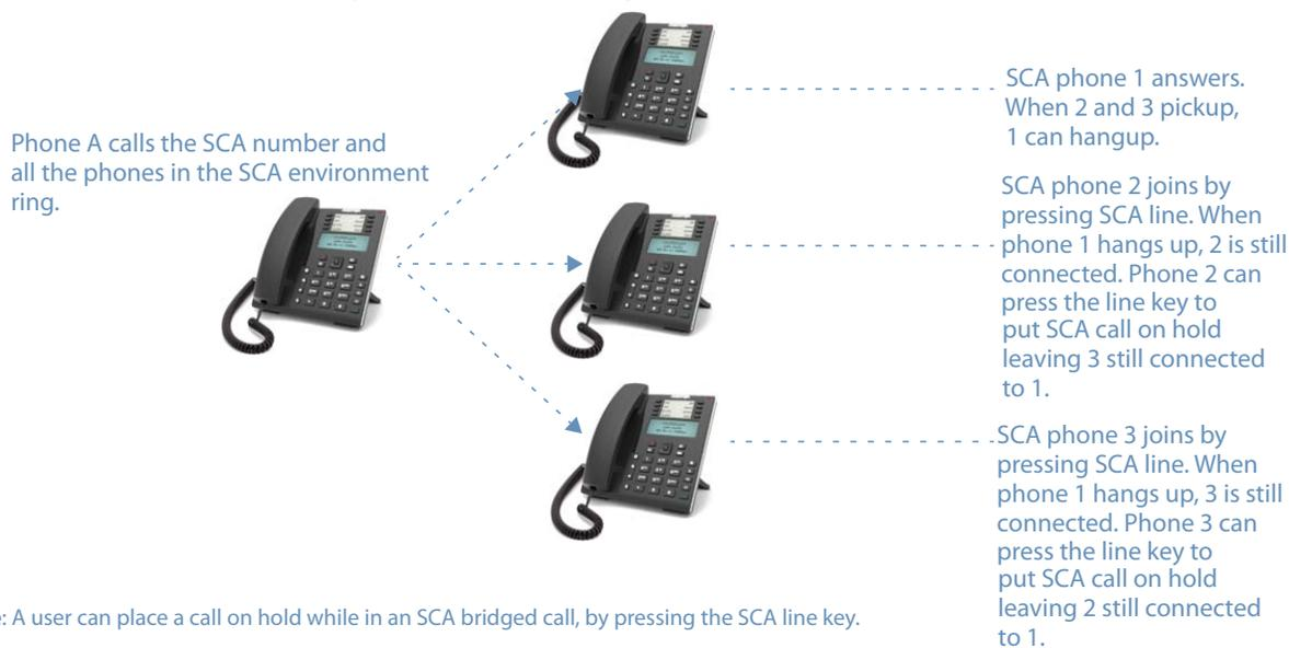
Using the example above, when a call comes into Phone 1, Phone 2 and Phone 3 can pickup the same call by pressing the SCA line key. Phone 2 and 3 display the call they are bridging into on the LCD of the phones. Existing SCA parties in a bridge or one-to-one call hear an audible beep when another party has joined the call.
