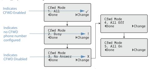
In this example, **CFWD All** is enabled as indicated by a check mark ( $\checkmark$ ), **CFWD Busy** is enabled but no call forward phone number is configured as indicated by a  $\frac{1}{4}$ , and CFWD No Answer is disabled, as indicated by an **X**.
