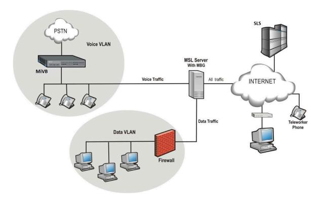
Figure 4: Server-gateway with Bridged Interface Configuration
