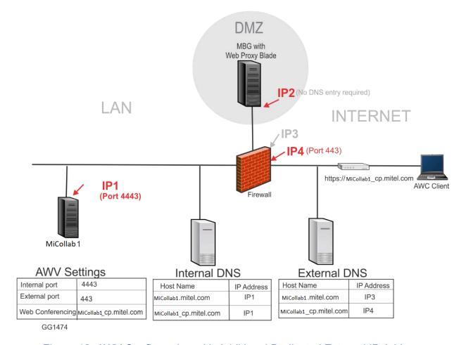
Figure 12: AWV Configuration with Additional Dedicated External IP Address
