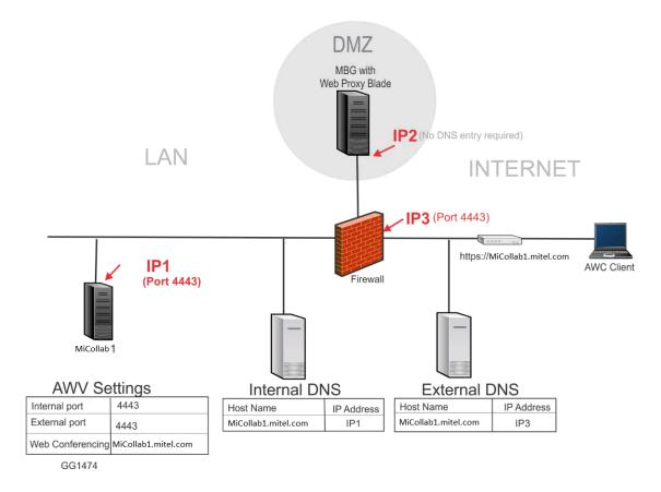
Figure 13: AWV Configuration with Dedicated TCP Port on Primary External IP Address
