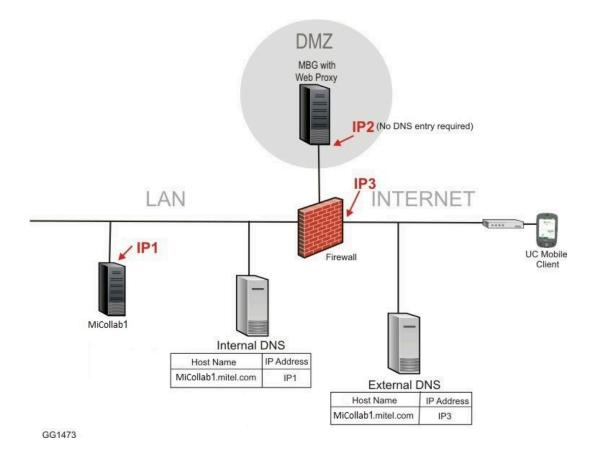
Figure 11: Basic DNS Configuration
