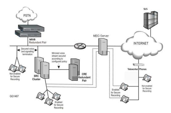
Figure 18: MBG Server with SRC Service (Direct Call Recording)
