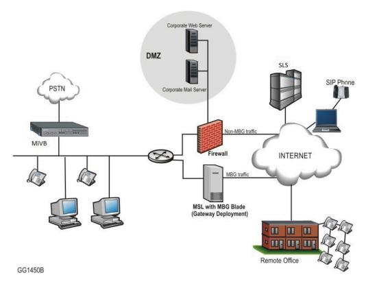
Figure 1: Server-Gateway Configuration
