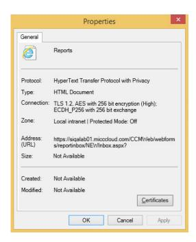
Figure 9: Page properties for CCMWeb showing TLS 1.2
