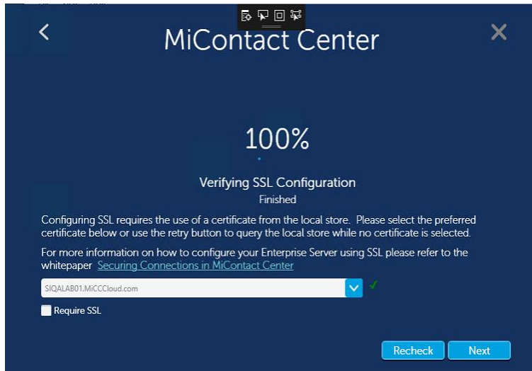
Figure 2: The SIQALAB01.MiCCCloud.com certificate has been used to configure IIS
