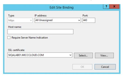
Figure 5: Sample completed site bindings configuration
