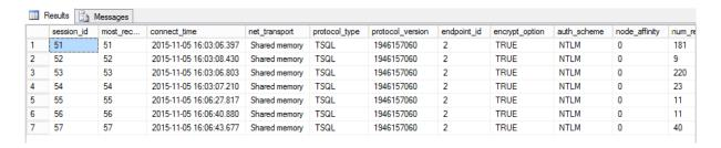
Figure 15: Sample query output showing secured connections
