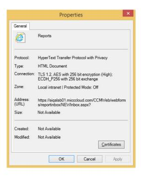
Figure 9: Page properties for CCMWeb showing TLS Connection
