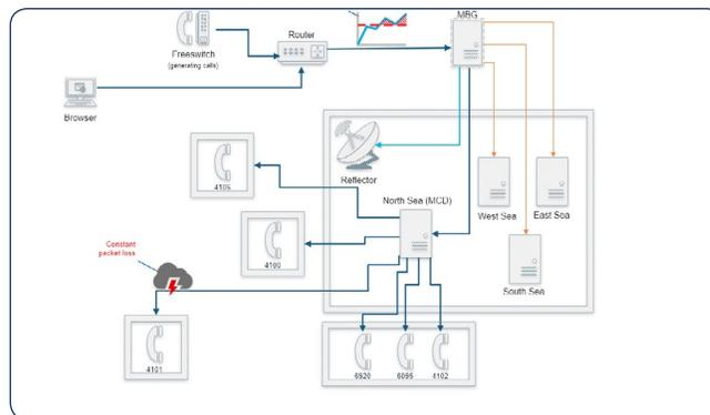
If your network diagram is valid, Mitel Performance Analytics overlays health status icons over the devices being monitored. The health status icons are linked to the alarm filter, just like the Location Map panel, the Alarms panel, and the device hierarchy at the left of the dashboard.
