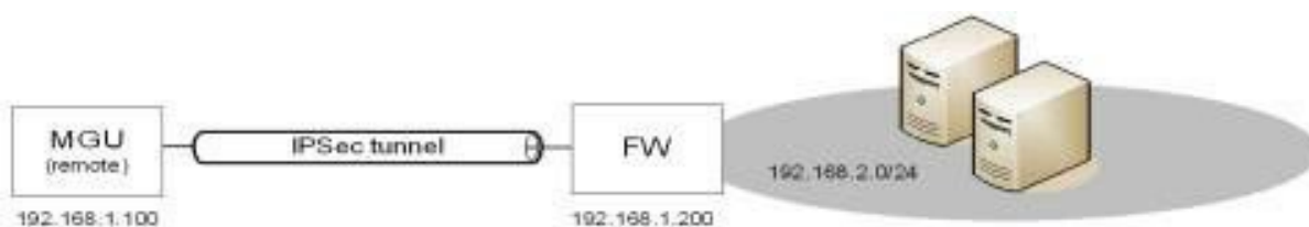
Figure 13: IP communication between MGU2 and a remote IPsec peer
