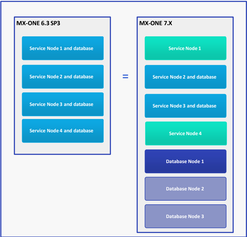
Figure 25 - Hybrid scenario - Four Service Nodes
