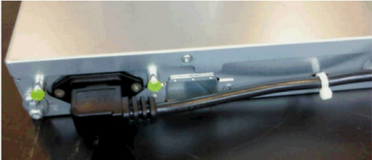
Figure 2.30: Secure Main cables
