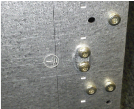
Figure 2.19: Earthing point 7U-chassis
