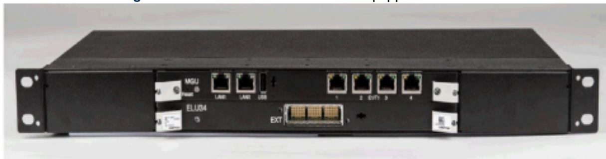
Figure 2.1: The MX-ONE 1U chassis equipped with MGU2 and ELU34
