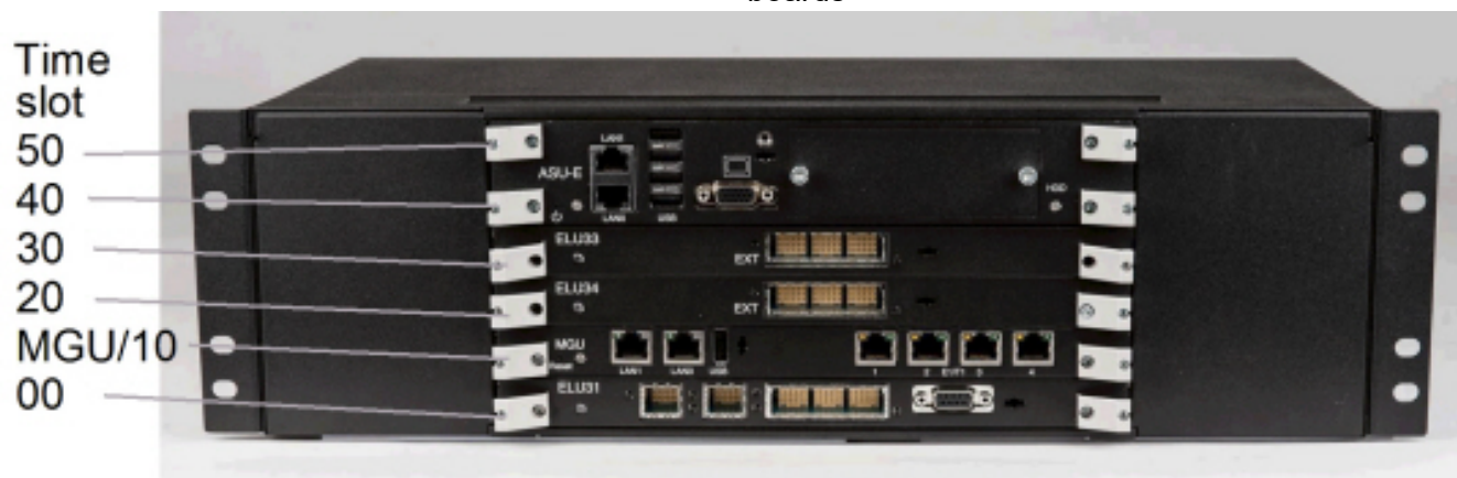
Figure 2.2: MX-ONE Lite, 87L00039BAA-A, equipped with MGU2, ASU and 3 additional boards
