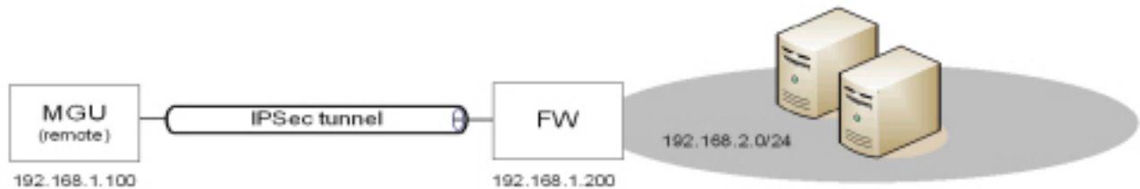
Figure 3.6: IP communication between MGU2 and a remote IPsec peer
