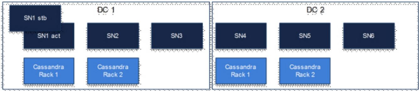
Figure 2.8: Cassandra in multi-site, co-located with the SNs, but only with one Cassandra node per DC. A total of 6 SNs and 6 DCs (geographical locations). No server redundancy.
