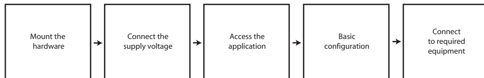
Figure 5. Recommended installation and configuration procedure
