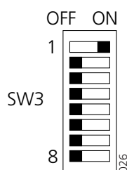
Figure 20: Setting the ELISE2 in Network Setup Mode.
