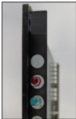
Figure 74: SLMAV8N, SLMAV24N – LEDs on the Front Panel
