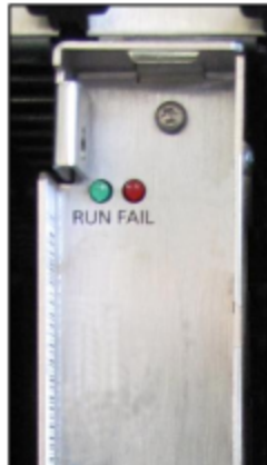
Figure 73: SLCN – LEDs on the Front Panel
