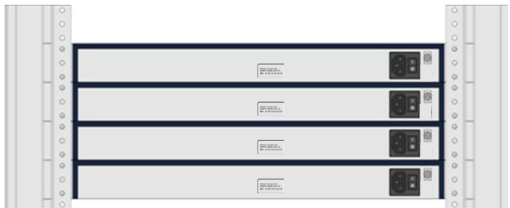
Figure 66: OpenScape Access system mounted in a 19"-rack (rear view)
