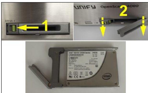
Figure 10: EcoServer: Replacing SSD Tray
