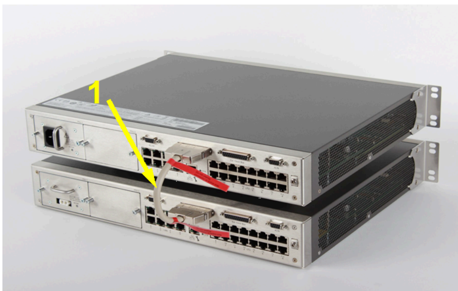
Figure 13: EcoServer: Duplex configuration with cross-connect cable (1)
