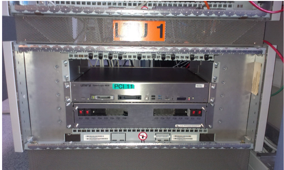
Figure 28: DC connection of EcoServer with DCDR (DC kit for 30" cabinet)
