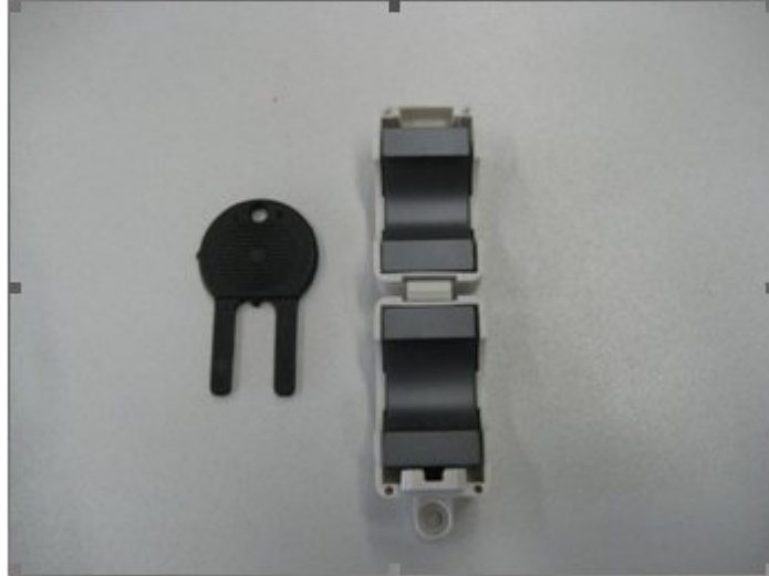
Figure 48: Key tool and opened ferrite core
