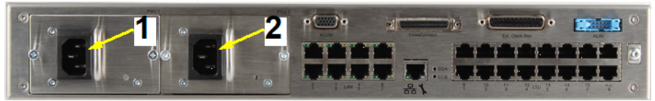
Figure 107: AC power supply for EcoServer
