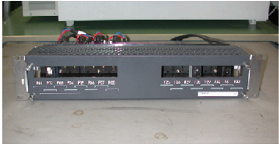
Figure 129: DCDR fuse unit for 19" installation
