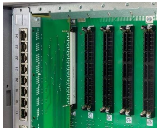
Figure 13: Patch-Panel with CHAMP-socket (NPPSC, S30807-Q6626-X)
