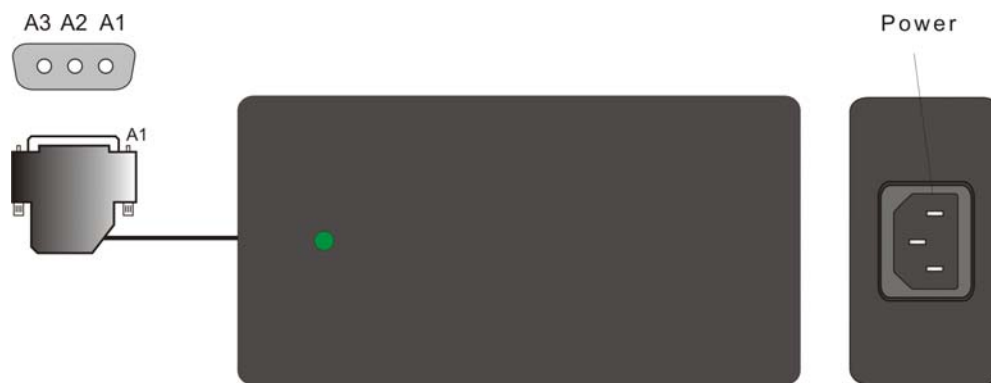
Image 3-19 AC/DC power supply unit
